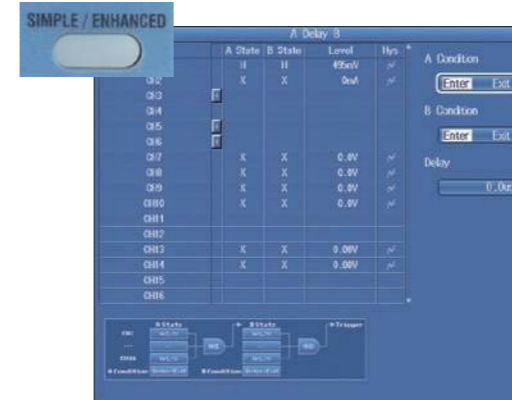
Example: "A delay B" trigger setup screen (After condition A becomes true, trigger the first time condition B becomes true after a set time has passed.)
