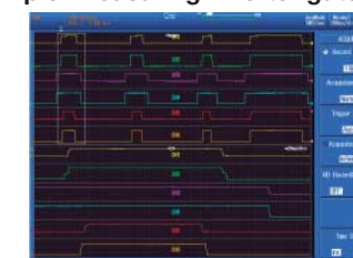
Example: Measuring inverter gate signals
