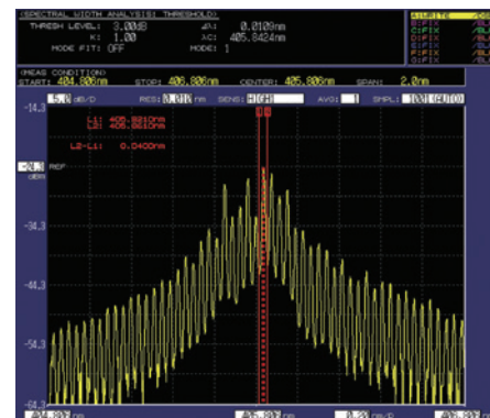
405 nm FP-LD measurement (resolution setting: 0.01 nm)
