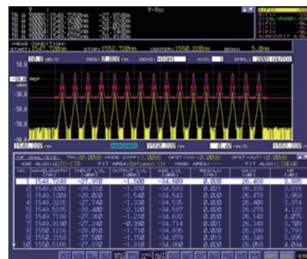
Figure 3 – The automated routine for the analysis of optical amplifiers provides a table with their relevant parameters
