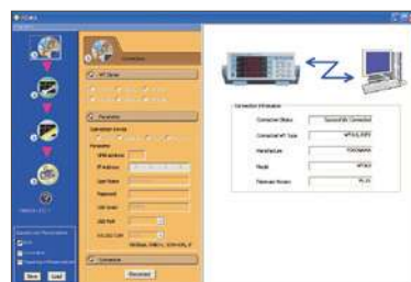
Configuring and Establishing a New Connection between the WT310E and a PC
