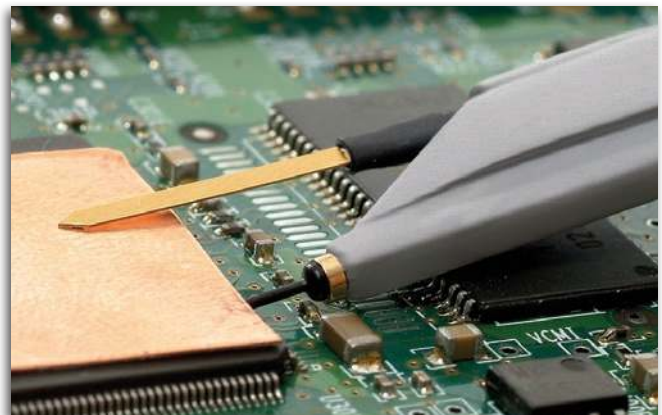
The Ground Blade and Copper Pad provide the shortest ground loop for excellent signal fidelity when probing an IC. Use them with the insulated IC Lead Tip to prevent shorting between test points.
