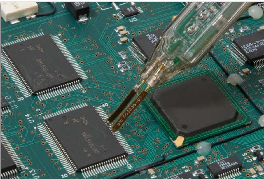
The IC leads with a compensation resistor provide excellent signal fidelity when probing pins of an IC. One side of each blade is insulated to prevent shorting the signal to the adjacent pin.
