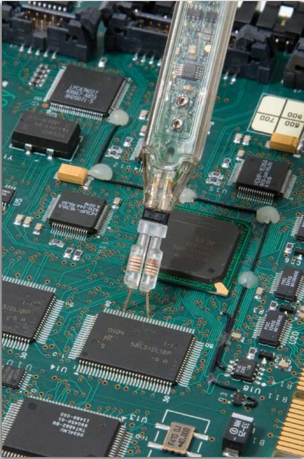
The Swivel Tip adapter can be adjusted to probe test points ranging from 0 to .300" apart with Z-Axis compliance.
