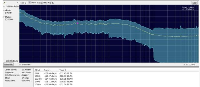
Phase noise and jitter measurements (Opt. 11) on the RSA5000 Series may reduce the cost of your measurements by reducing the need for a dedicated phase noise tester. Outstanding phase noise across the operating range provides margin for many applications. Here, phase noise on a 13 MHz carrier is measured at -119 dBc/Hz at 10 kHz offset. The instrument phase noise of < -134 dBc/Hz at this frequency provides ample measurement margin for the task.
