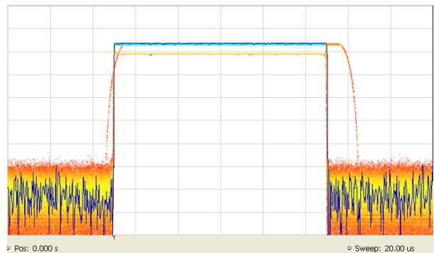
DPX Zero-span produces real-time analysis in amplitude, frequency, or phase vs. time. Up to 50,000 waveforms per second are processed. DPX Zero-span ensures that all time-domain anomalies are immediately found, reducing time-to-fault. Here, three distinct pulse shapes are captured in zero-span amplitude vs. time. Two of the three waveforms occur only once in 10,000 pulses, but all are displayed with DPX.
