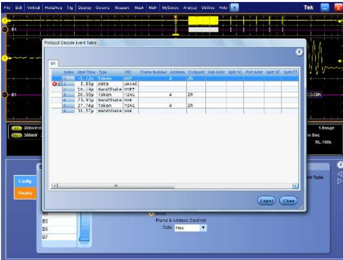
Event table showing decoded serial packet data in a long acquisition.
