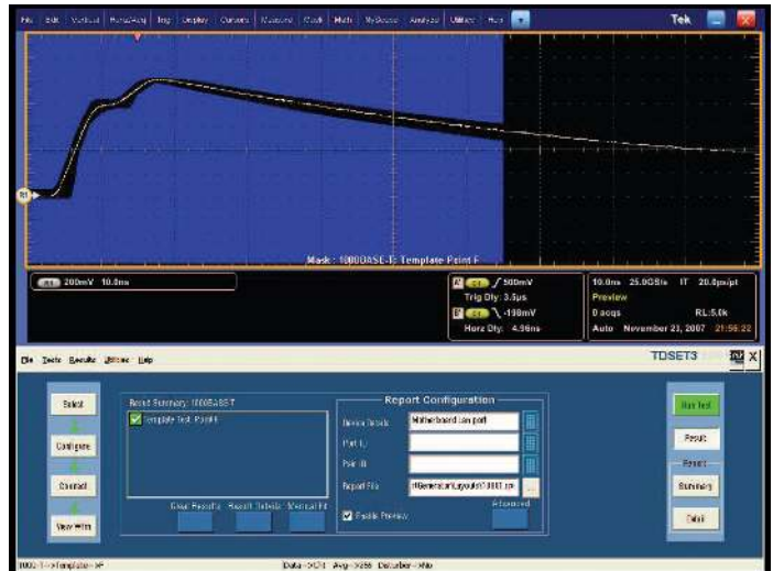
Ethernet Compliance Test Solution (Option ET3) – Receive full PHY layer support for Ethernet variants 10BASE-T, 100BASE-TX, and 1000BASE-T with the comprehensive, integrated Tektronix® Ethernet tool set. Analog verification, automated compliance software, and device characterization solutions are all included.
