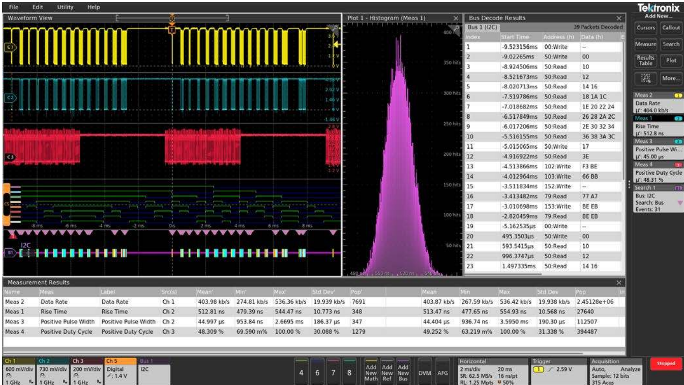
Figure 6: Viewing three analog channels, eight digital channels, a decoded serial bus waveform, decoded serial packet results table, four measurements, a measurement histogram, measurements results table with statistics and a search on serial bus events - simultaneously!
