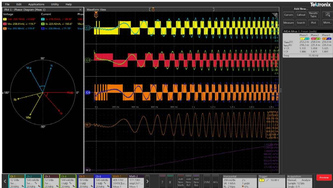
Figure 31: On the left is a Phasor diagram displaying the phase and magnitude of current and voltage measurements for all three phases of power. In the results badge on the right, are the results from the automated measurements of power quality.
