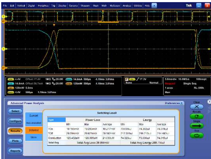
Switching Loss measurements.
