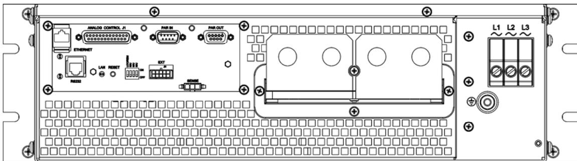
**Figure 3-5. SG Rear Panel with Ethernet Option (10V-30V)**
