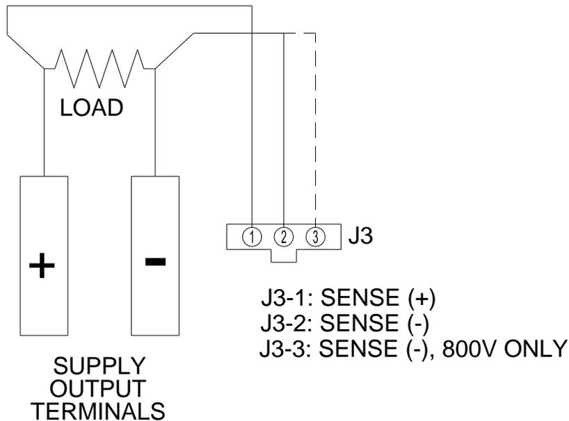
**Figure 3-14. Remote Sensing Operation at the Load**
