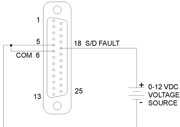
**Figure 3-19. Remote Shutdown Using DC Voltage Source**
