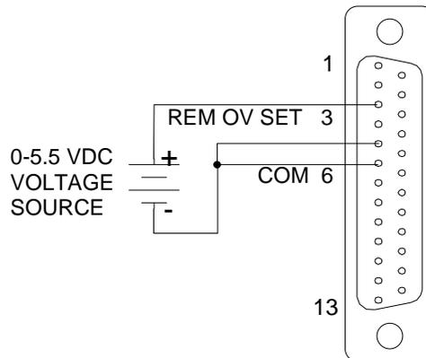
**Figure 3-18. Remote Overvoltage Set Using DC Voltage Source**
