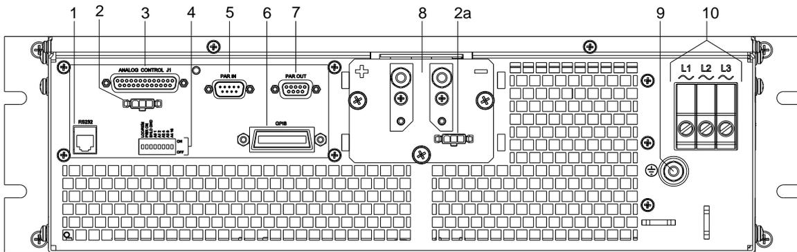
**Figure 3-2. SG Rear Panel with GPIB Option (40V-800V)**
