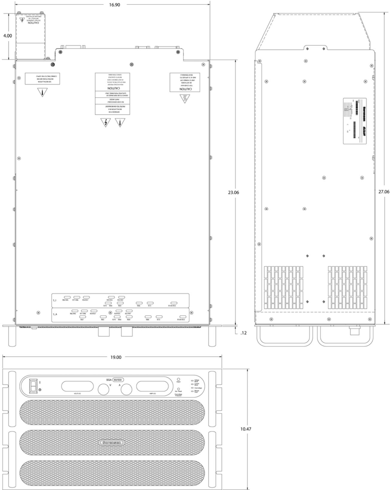
Figure 2-4. SGA Dimensions, 6U Models, 20kW to 30kW
