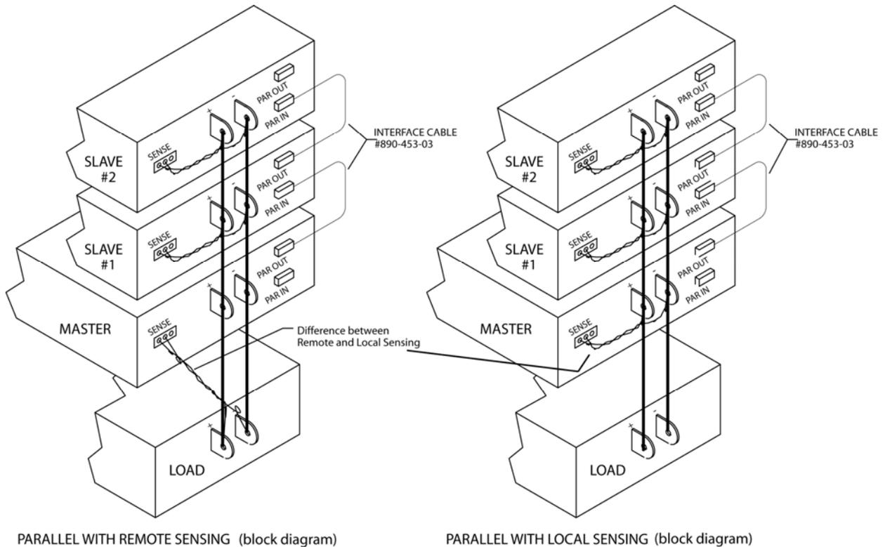
NOTE: The voltage display on the slave units will be slightly higher than the master unit. The twisted pair cable length must be as short as possible.
