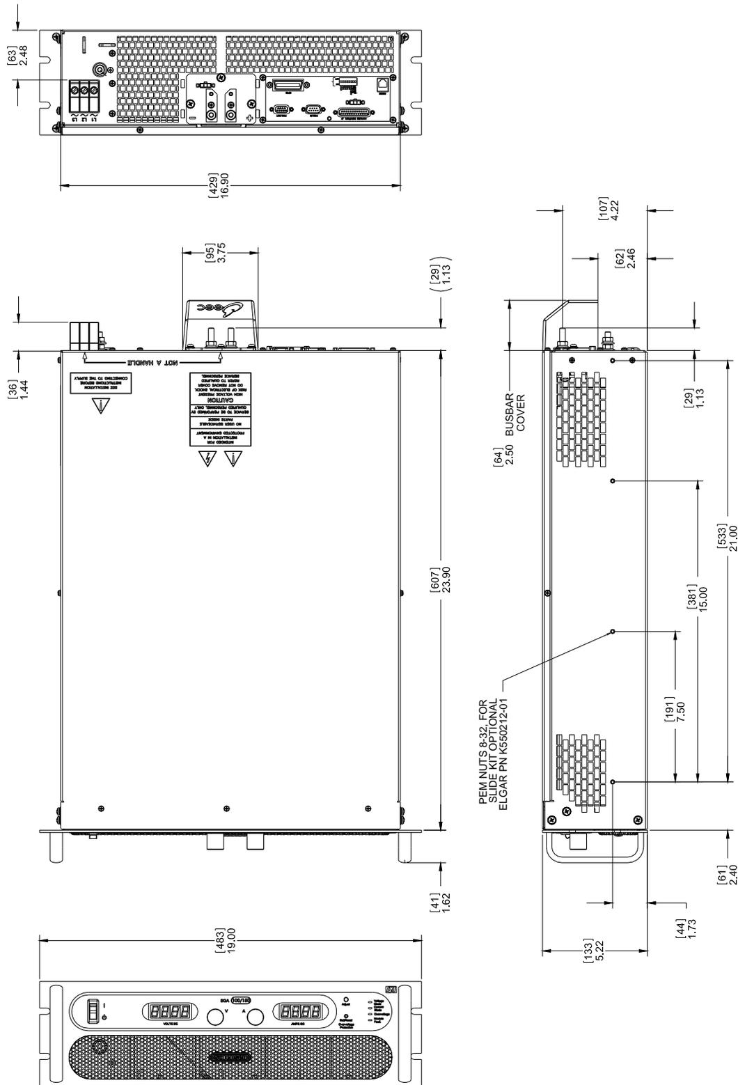
Figure 2-10 SGA 800V Detailed Chassis Dimensions for Installation
