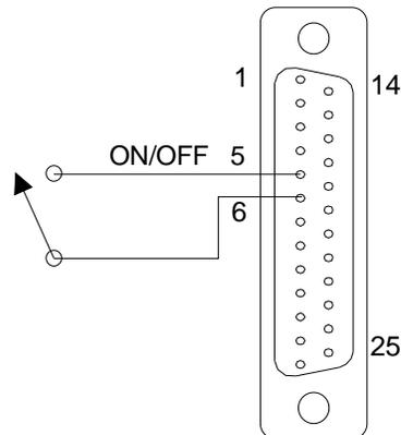
**Figure 3-15. Remote Output ON/OFF Control by Contact Closure**
