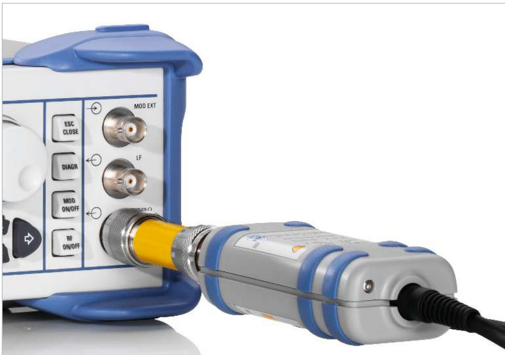
The R&S®SMB100A with connected R&S®NRP-Z92 power sensor performs automatic level correction.
