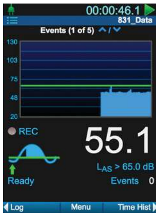
A recording icon (●) will turn red on the Model 831C display when recordings are being made.
