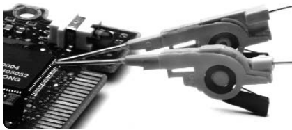
Figure 9.2. Extremely small-sized clips for probing PQFP and SOIC SMT packages.
