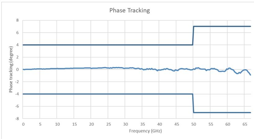
Figure 18. 11667D phase tracking versus frequency (typical)
