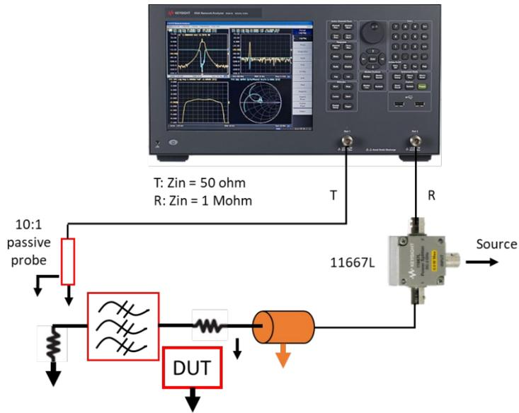
Figure 3. Non- 50-ohm LF filter measurement
