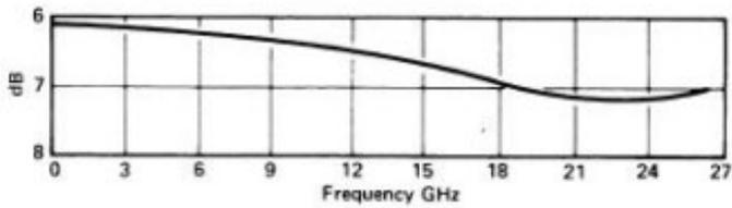
Figure 12. 11667B Insertion loss versus frequency (typical)
