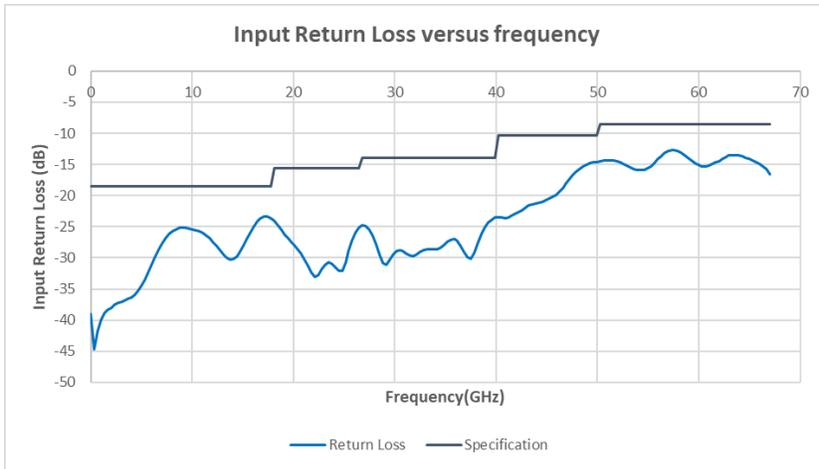
Figure 14. 11667D Input return loss versus frequency (typical)
