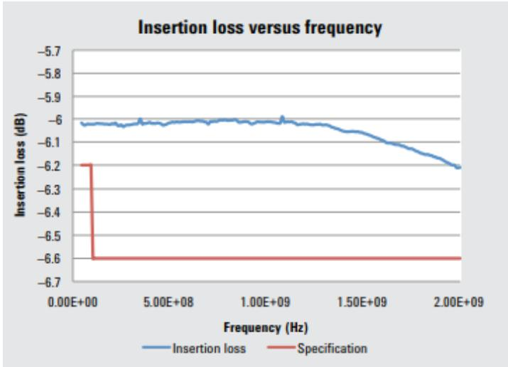
Figure 8. 11667L insertion loss versus frequency (typical)
