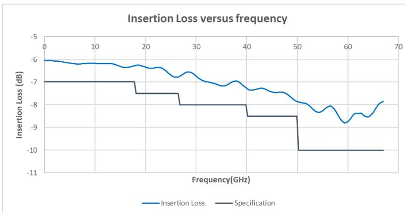
Figure 16. 11667D Insertion loss versus frequency (typical)
