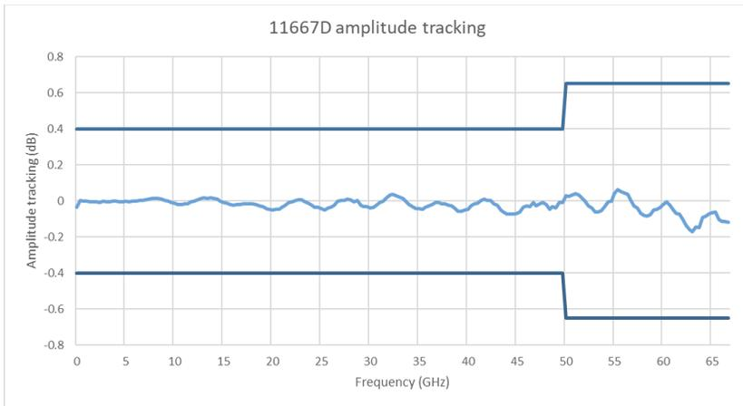
Figure 17. 11667D Amplitude tracking versus frequency (typical)
