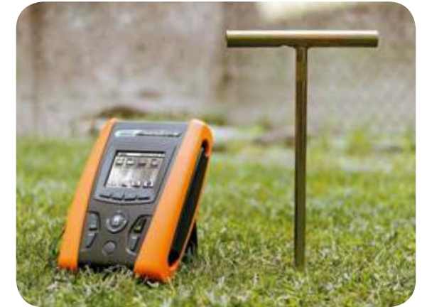
Earth resistance measurement by Volt-ampere method
