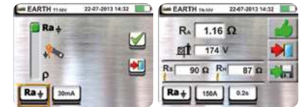
Earth resistance measurement by Volt-ampere method
