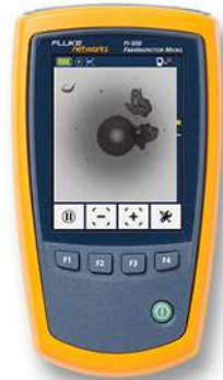
FI-500 displaying a dirty fiber endface
