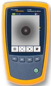
FI-500 displaying a clean fiber endface
