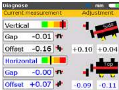
3. Corrective action using the Fluke 830 Laser Shaft Alignment.
