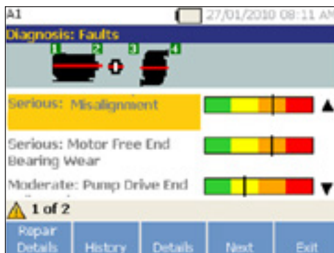
2. Diagnosis and repair recommendation using the Fluke vibration tool.
