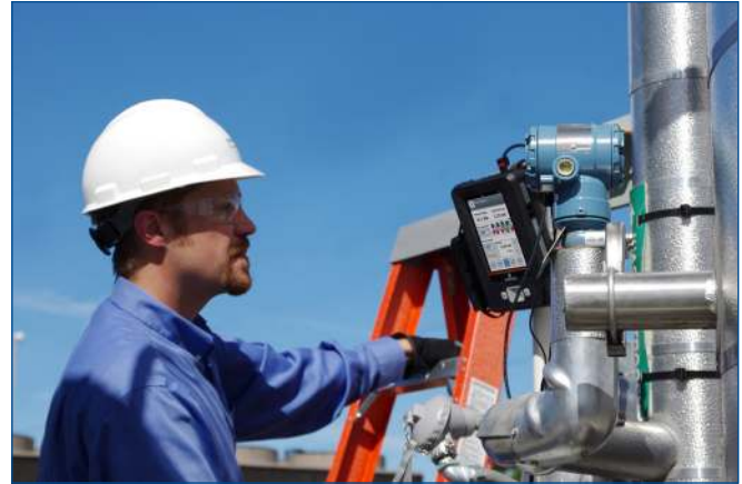
The magnetic hanger accessory allows you to attach the Trex unit to a pipe, freeing up your hands for other work.
