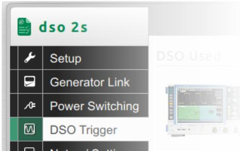
A DSO module is available to extend the basic TEMA3000 software package. DSOs with Ethernet and USB interfaces can be controlled from TEMA3000 software. Apart from setting timebase and amplitude, measurement features in the DSO can also be accessed and measurement results added to the test report. Tektronix, Keysight, Lecroy and Rohde & Schwarz models are supported as standard.
