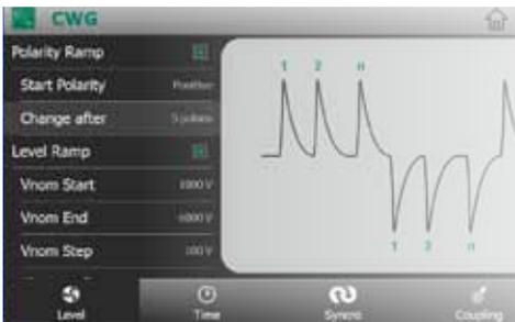
Connected using the Ethernet cable to AVI3000, TEMA3000 opens a window which emulates the EPOS in AVI3000. All parameters are input exactly as on the AVI3000 front panel. Any generator connected to TEMA3000 will be simultaneously programmed over the Ethernet cable. Conversely, parameters entered on AVI3000 are changed in TEMA3000.
