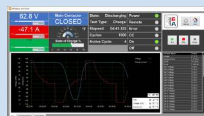
Results display screen showing voltage, current, and the results of a capacity simulation test.
