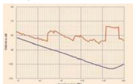
A competitive instrument lacking a DSP analyzer produces false THD+N readings (red trace) from a popular A/D converter; but both the ATS-1 Dual Domain and the Audio Precision 2700 Series graph the true performance of the converter (from 5 dB to 28 dB lower), as shown by the blue trace.
