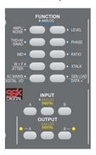
and make the measurement. Selection of analog and digital inputs is clearly indicated on the front panel with LED legends. ATS-1 makes graphs of swept measurements in real time
