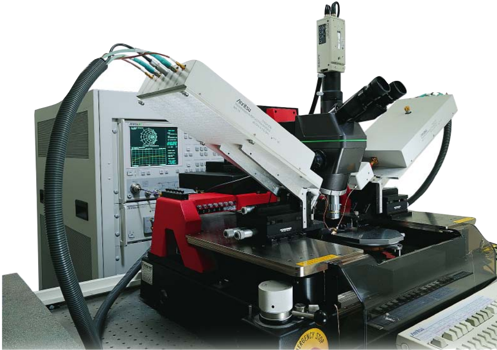
On-wafer measurements to 110 GHz with the ME7808B
