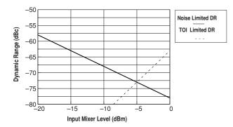
Agilent 8563E-K35: Typical W-CDMA ACPR Dynamic Range (measured in a 4.096 MHz integration BW)
